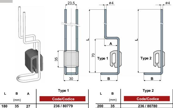
MATERIALS: Support elements made out of stainless steel AISI 304, body of coupling made out of reinforced polyamide.
